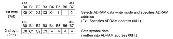
To specify symbol data continuously to the next address, specify only symbol data as follows. The address of ADRAM is automatically incremented. Specification of addresses is therefore unnecessary.
