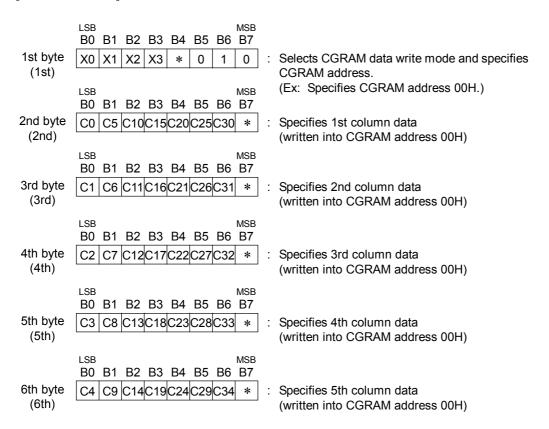
To specify character pattern data continuously to the next address, specify only character pattern data as follows. The addresses of CGRAM are automatically incremented. Specification of an address is therefore unnecessary. The 2nd to 6th byte (character pattern data) are regarded as one data item, so 250 ns is sufficient for  $t_{DOFF}$  time between bytes.
