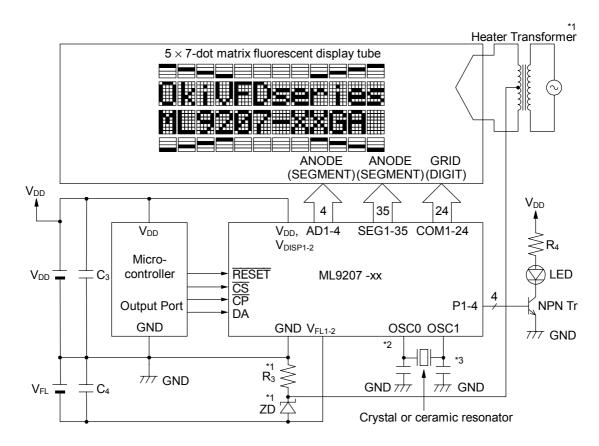
Notes: \*1. The application circuit indicates a circuit by which fluorescent display tube filaments are ac driven using a heater transformer. Contact fluorescent display tube manufacturers for the methods and circuits of driving fluorescent display tube filaments.
