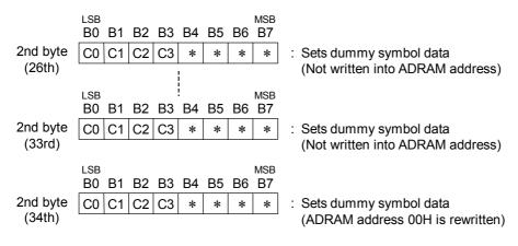
X0 (LSB) to X4 (MSB) : ADRAM addresses (5 bits: 24 characters) C0 (LSB) to C3 (MSB) : Symbol data (4 bits: 4-symbol data per digit)
